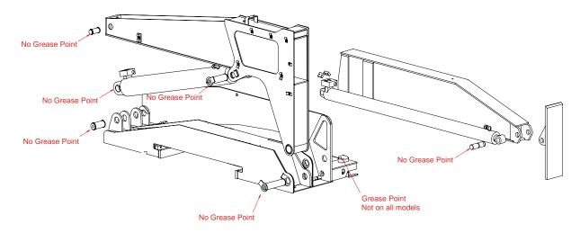
NB: Do not use Molybdenum Disalphide grease as it reacts with the glacier bearing
