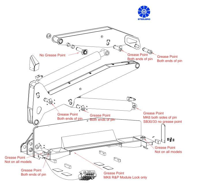
NB: Do not use Molybdenum Disalphide grease as it reacts with the glacier bearing
